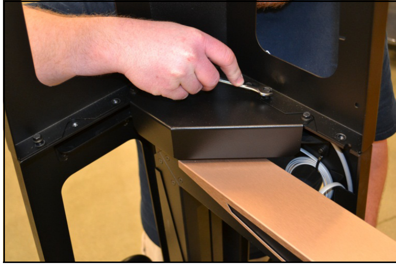
Figure 4 Top Sensor Support Attached
