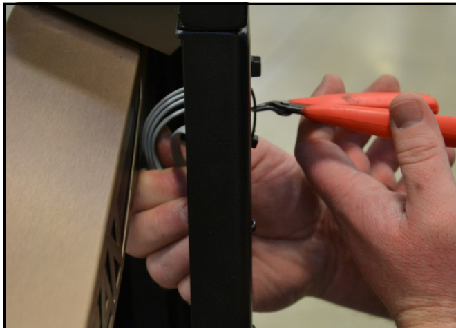
Figure 5 Location of Height Sensor Cable
