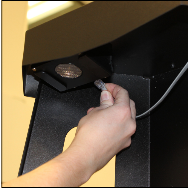
Figure 8 Connecting the Height Sensor Cable
