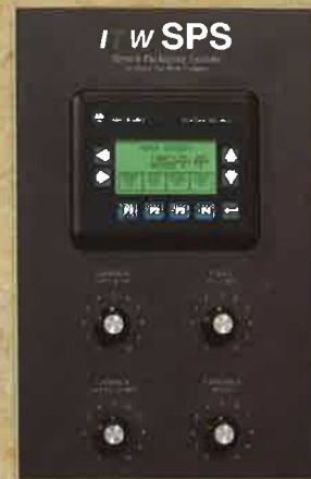
Allen Bradley PLC with Panel View operator interface.
