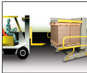
2. Place loaded pallet into rotator/inverter.
