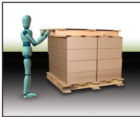
1. Add replacement pallet or slip sheet to top of load.
