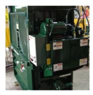
The side-mounted, self-contained power unit is convenient for maintenance and servicing. Front opening control panel eliminates the need for 48" side clearance as required by NEC standards.
