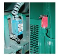
A redundant interlock system is incorporated into the feed-gate switch.
