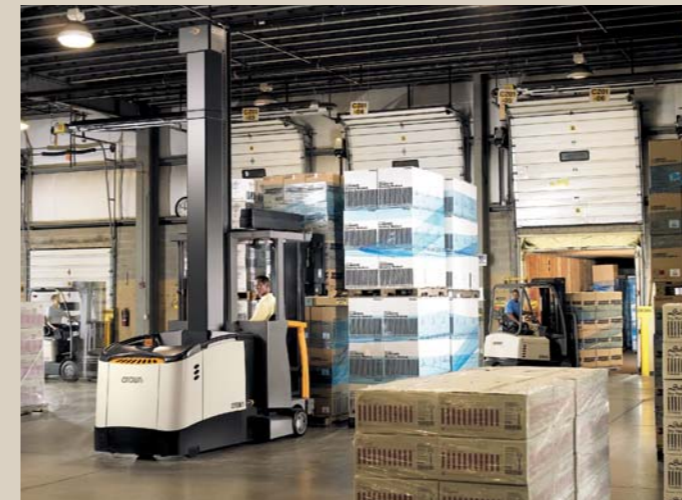
STAGING: Another operational advantage of the TSP 6000 Series, with its compact three-wheel design providing excellent maneuverability and a tight turning radius to help the operator easily transport and position full pallet loads.
