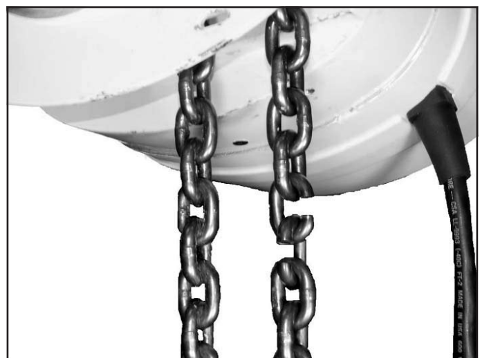
Figure 5-4. Installing Coil Load Chain Using Two "C" Links (1/4, 1/2 & 1 ton hoists)
