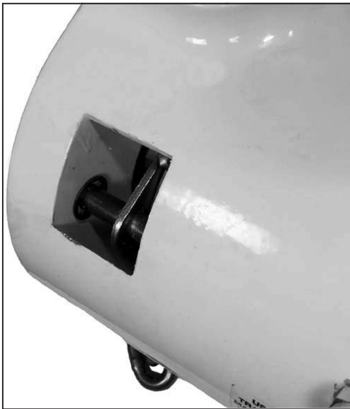
Figure 7-13. Removing Chain Guide Support Pins
