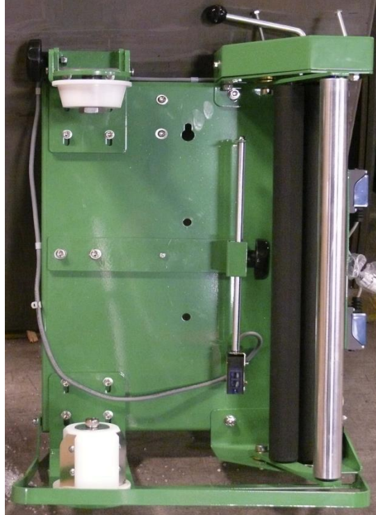
Figure 3: Bracket in the Shipping Position
