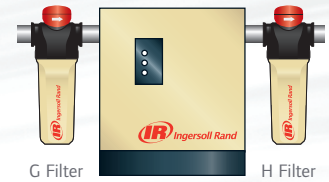
G Filter Refrigerated Dryer H Filter
